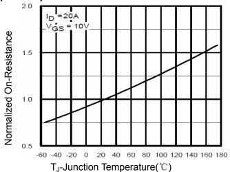
Figure 4 Rdson-JunctionTemperature
