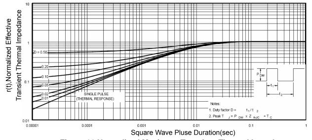
Figure 11 Normalized Maximum Transient Thermal Impedance
