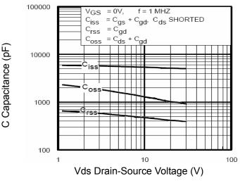
Figure 7 Capacitance vs Vds
