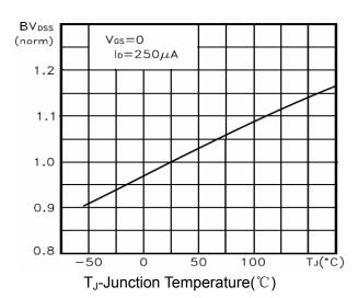
Figure 9 BV<sub>DSS</sub> vs Junction Temperature
