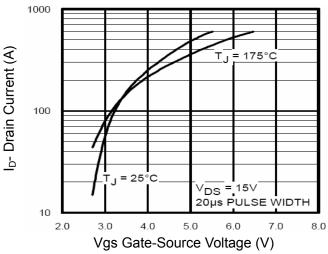
**Figure 2 Transfer Characteristics**
