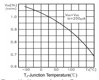
Figure 10 V<sub>GS(th)</sub> vs Junction Temperature
