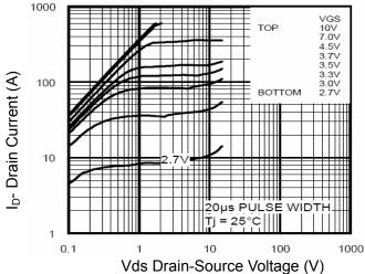
**Figure 1 Output Characteristics**
