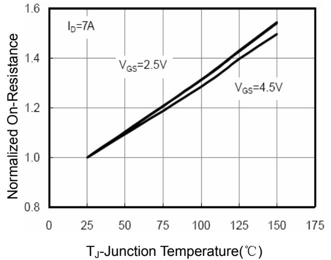
Figure 8 Drain-Source On-Resistance
