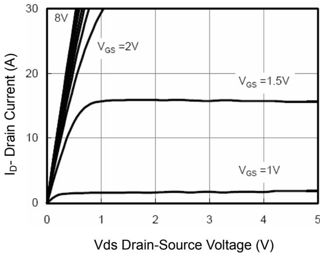
Figure 5 Output Characteristics
