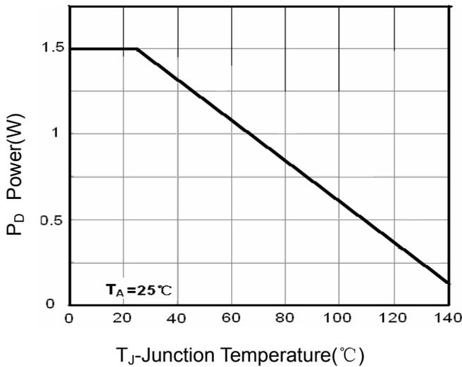
Figure 3 Power Dissipation
