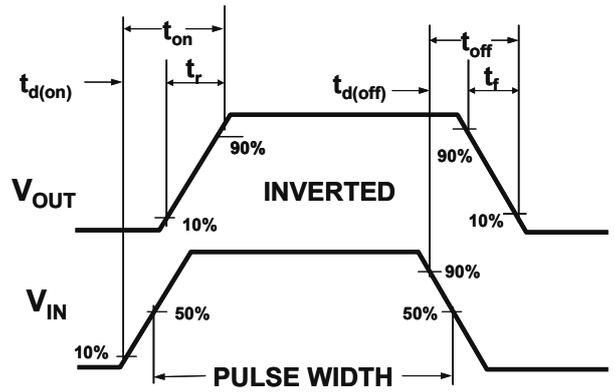
Figure 2: Switching Waveforms
