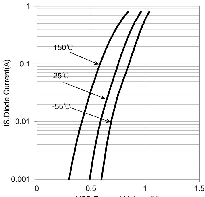
Body Diode Forward Voltage
