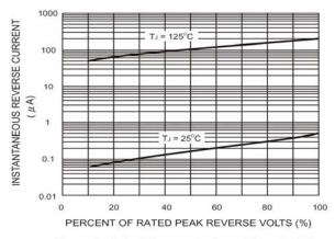
Figure 4. Typical Reverse Leakage Characteristics Per Bridge Element
