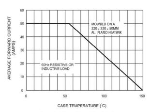
Figure 1. Forward Current Derating Curve
