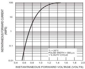
Figure 2. Typical Instantaneous Forward Characteristics Per Brdige Element
