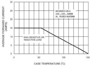
Figure 1. Forward Current Derating Curve
