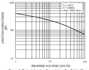
Figure 5. Typical Junction Capacitance Per Bridge Element
