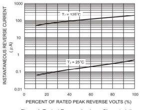
Figure 4. Typical Reverse Leakage Characteristics Per Bridge Element
