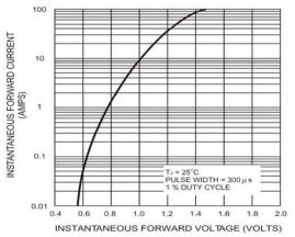
Figure 2. Typical Instantaneous Forward Characteristics Per Bridge Element
